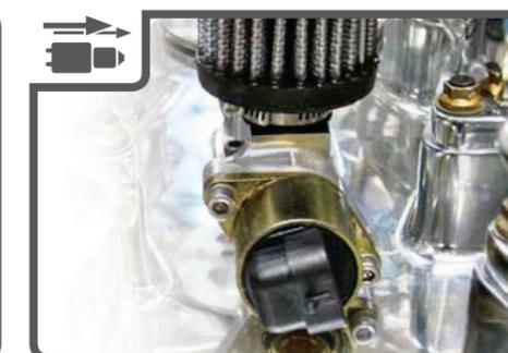
Provides the extra air needed to meet the demands power steering & air conditioning put on your engine. Also increases cold start RPM.
